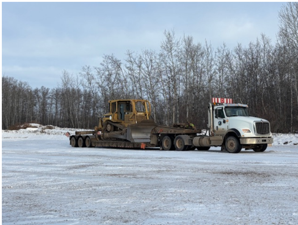
PW Figure 0.04. Lowboy Hauling Dozer to Stockpile Site
